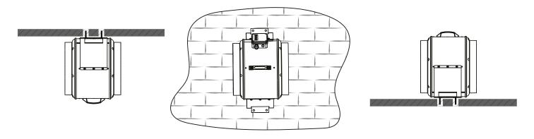
Connect the air ducts of the appropriate diameter to the fan (connections must be airtight).
