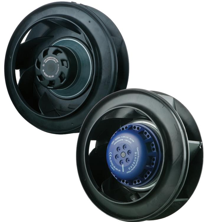
The Frigate ERV/HRV 80/150 units are equipped with supply and exhaust centrifugal fans with backward curved blades and build-in thermal overheating protection with automatic restart. The electric motors and impellers are dynamically balanced.
