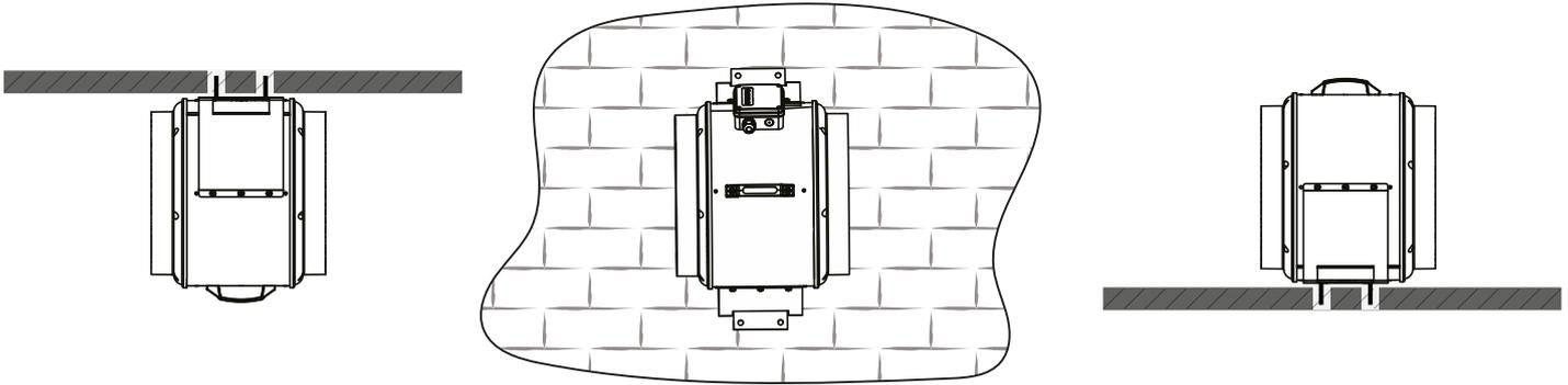
Connect the air ducts of the appropriate diameter to the fan (connections must be airtight).
