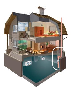
The **VENTS VK-AntiRADON** fan is fixed on the wall. The polluted air is extracted at roof level. The air ducts must be located at least 10' away from any window.
