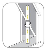
For airtight installation of **VK-AntiRADON** fan rubber collars with stainless clamps are recommended to use. \* not supplied with the fan
