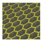
The high-tech ceramic regenerator with heat recovery efficiency up to 70 % is used for heating of supply air by means of the exhaust air heat recovery. Due to its honeycomb structure, the unique heat exchanger has larger air contact area and excellent heat conducting and accumulating properties.
