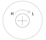
Turn the screw clockwise **(towards the L)** to increase the sensitivity of the pressure switch. Turn one half to one full turn. Continue turning until the correct calibration for dryer is achieved.
