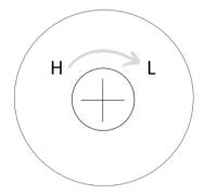
Turn the screw counter-clockwise (towards the H) to reduce the sensitivity of the pressure switch. Turn one half to one full turn. Continue turning until the correct calibration for dryer is achieved.
